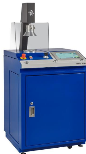
Fig.15. – Stand de testare la aerosoli - TSI CERTITEST 8130A/ AUTOMATED FILTER TESTER model 8130A/EN
